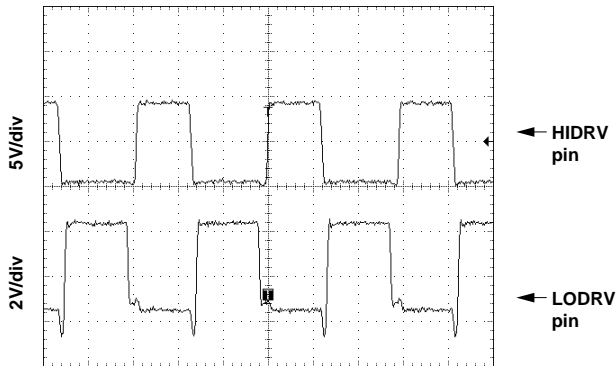
Switching Waveforms, 9A Load
